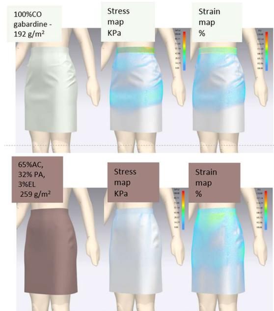
Figure 8: Simulated results with stress and strain maps for a skirt in different fabrics.
