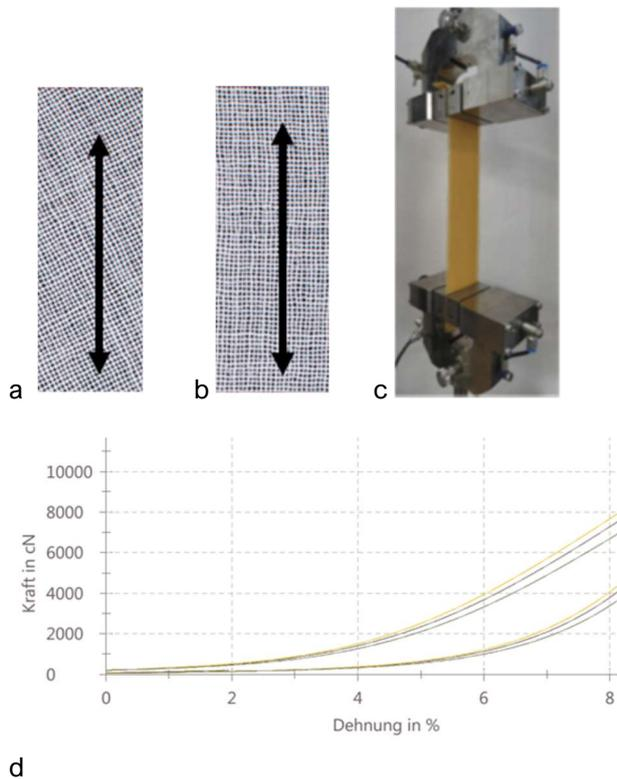
Figure 10: Tensile and shear elongation in (a) warp and (b) bias direction (c) ZwickRoell tensile test device and (d) elongation/force curve.
